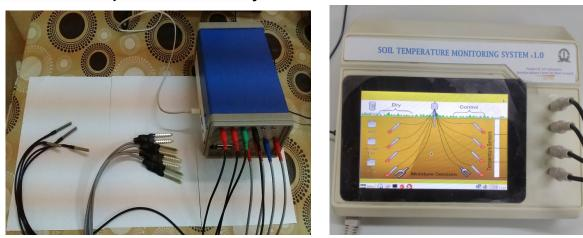
Multi-Channel IoT enabled soil moisture measurement system v1 & v2
