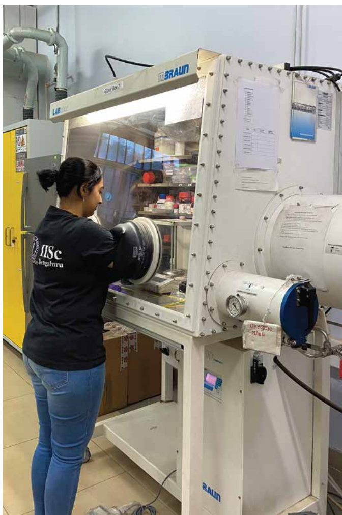
Akshatha Venkatesh from Aninda Bhattacharyya's lab assembling a lithium-ion battery in the glovebox under inert conditions
