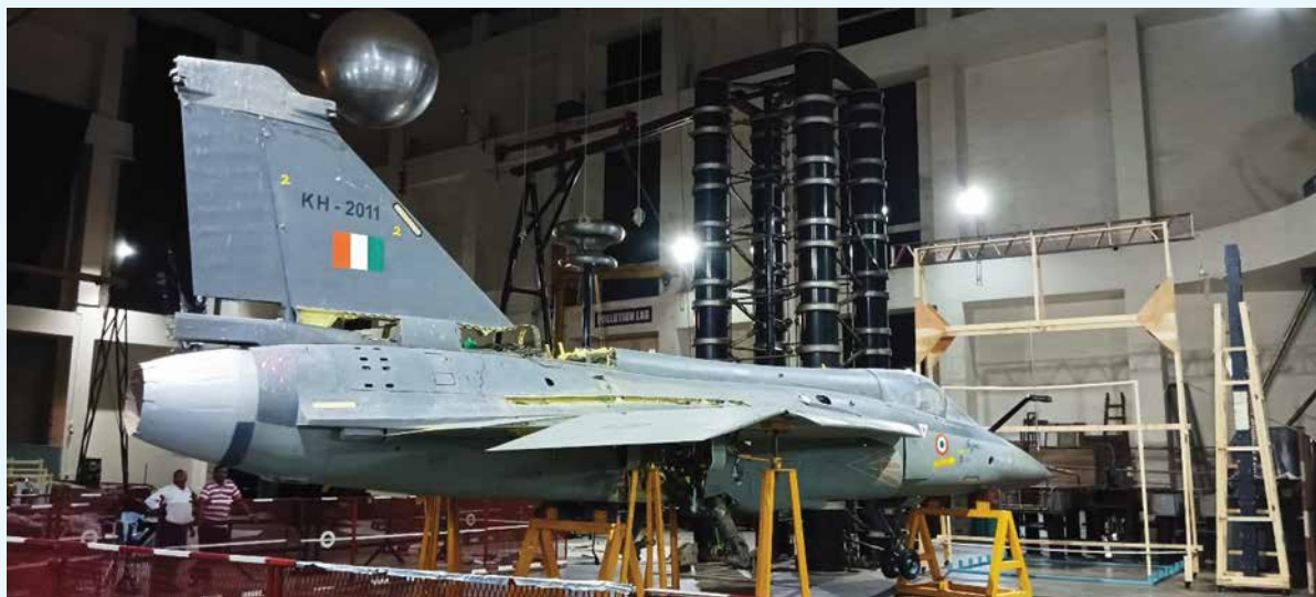
LCA outer shell being tested in the High Voltage Laboratory
