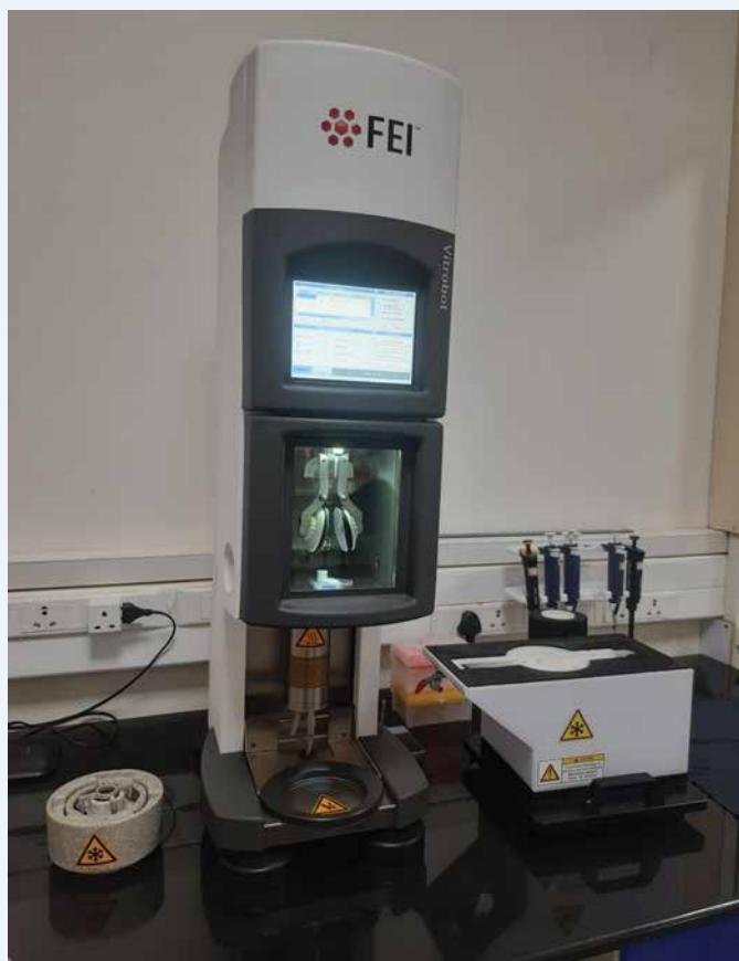
A modern plunge freezer device for flash freezing Cryo-EM samples at the Advanced Centre for Cryo-Electron Microscopy, IISc
