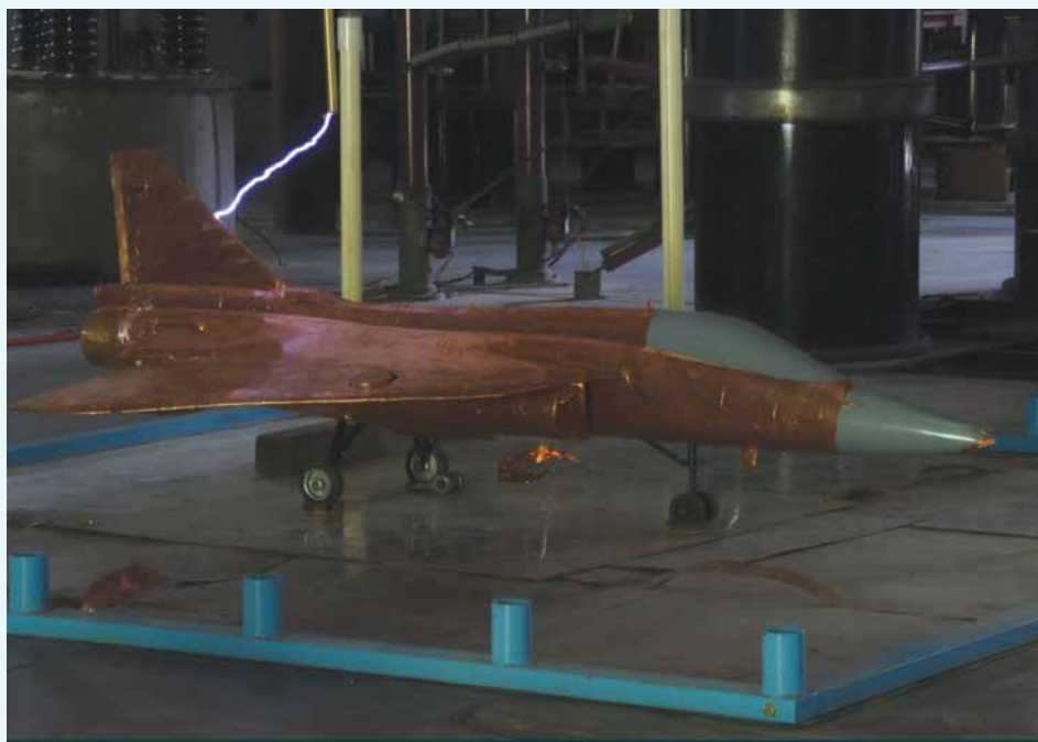
Simulation of lightning attachment to scaled version of LCA
