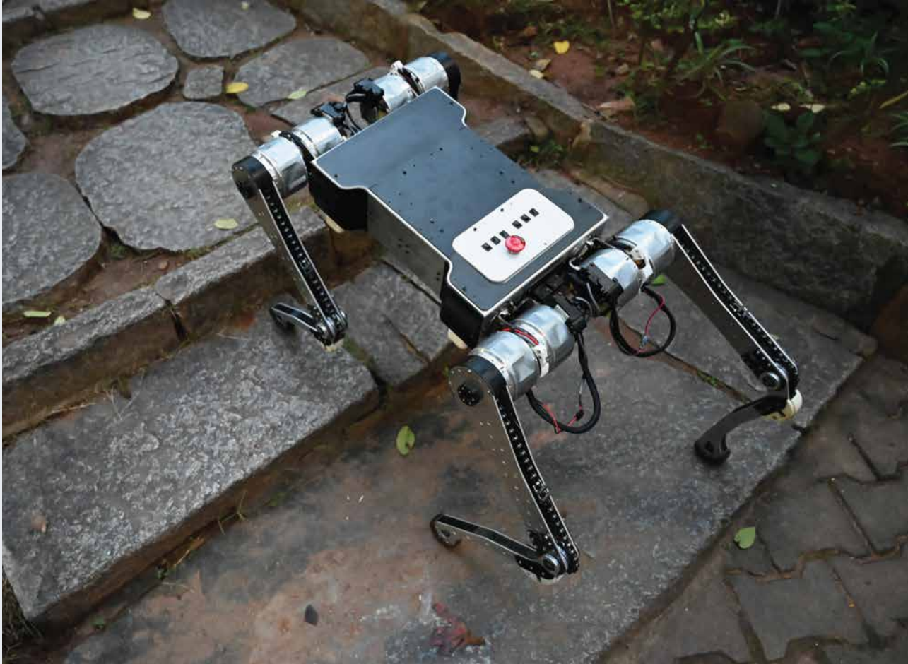
Legged robots like Stoch are meant for use in applications that require locomotion over unstructured and rough terrain
