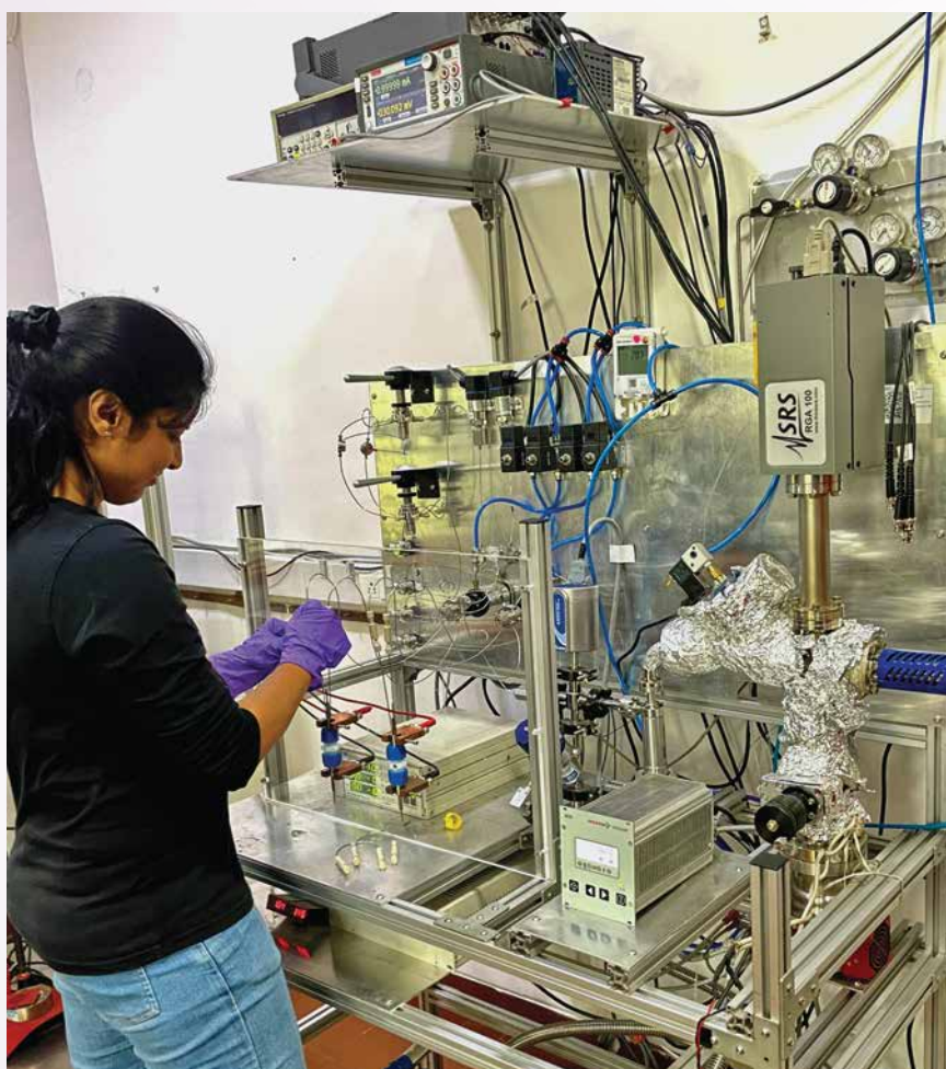
Akhila S from Naga Phani Aetukuri's lab setting up batteries on a differential electrochemical mass spectrometer
