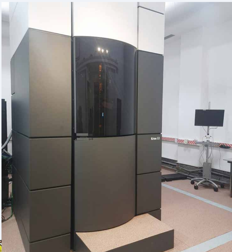
A 300kV transmission electron microscope used in NCBS for Cryo-EM
