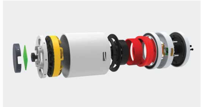
Exploded view of fully integrated robotic joint actuator
